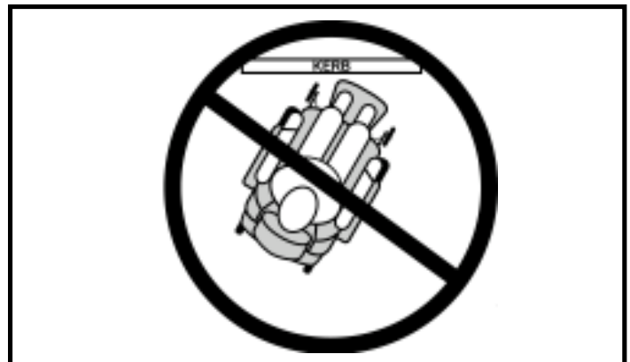
Figure 3. Incorrect Kerb Approach
