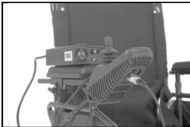
Figure 22. Charging the Batteries
