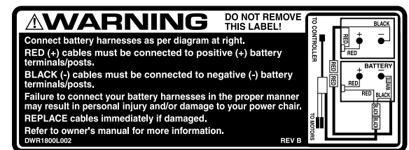
Figure 37. Battery Wiring Label
