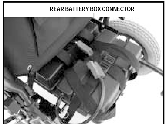
Figure 7. Rear Battery Box
